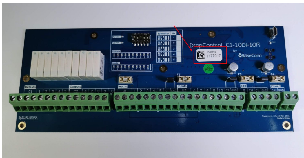
PCB ID MOD10DI-10R with a label specifying its serial (e.g. PCB ID 1177017)
